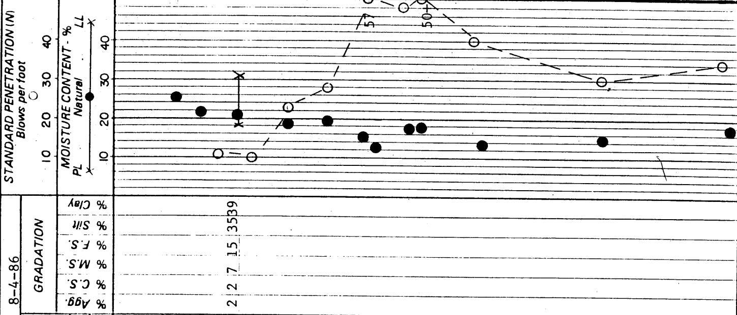
Dense dark gray fine to coarse SAND and SILT (SM), trace gravel. Damp.
