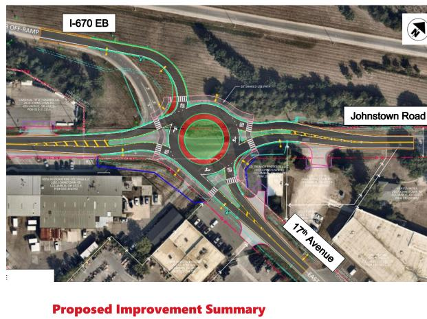
o Replace the existing stop controlled skewed intersection of Johnstown Road, 17<sup>th</sup> Avenue and I-670EB Exit Ramp with a single-lane roundabout.
