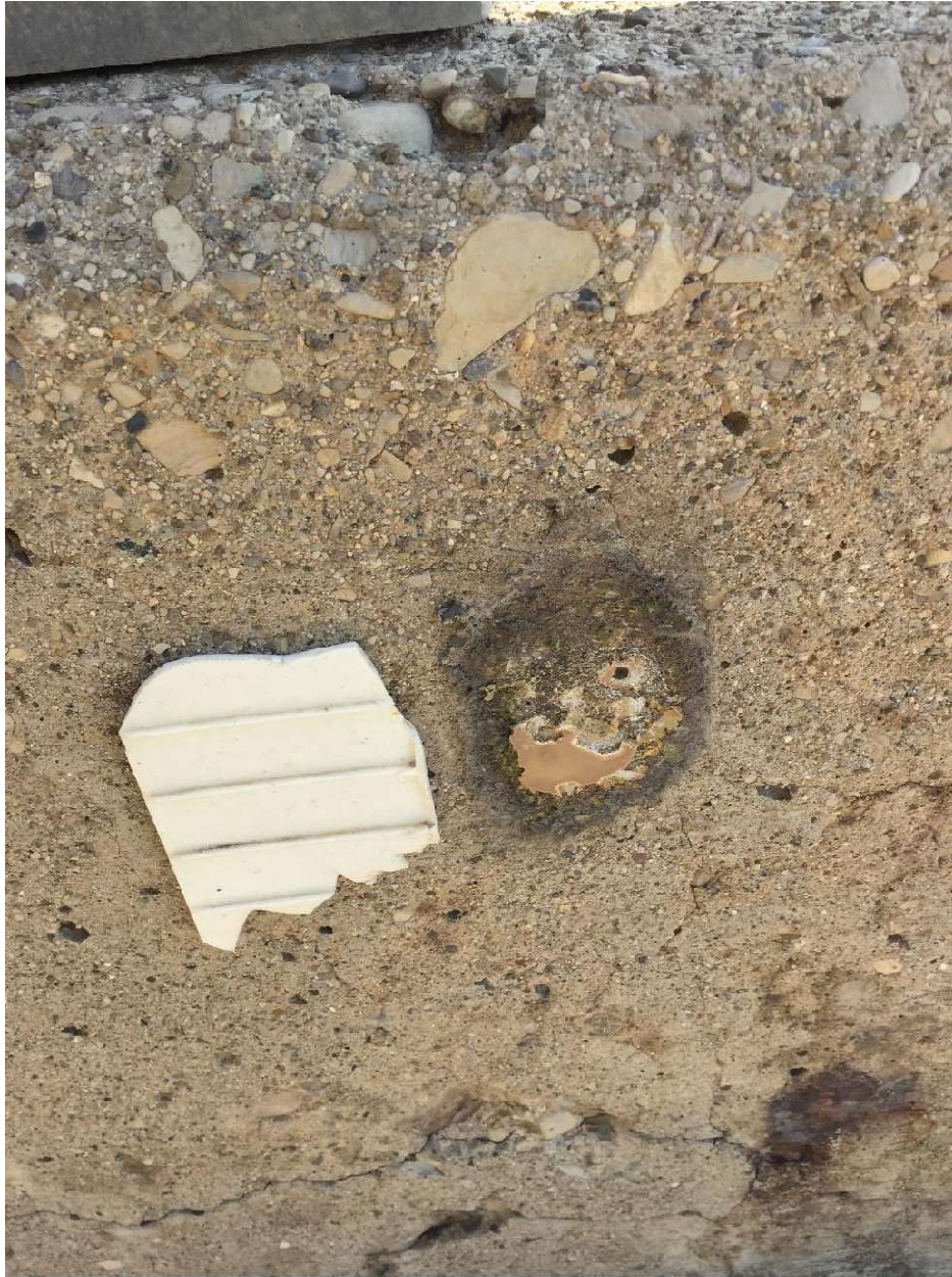
Photo #1: View of HA #1 - Non-asbestos-containing reflective panel caulking.
